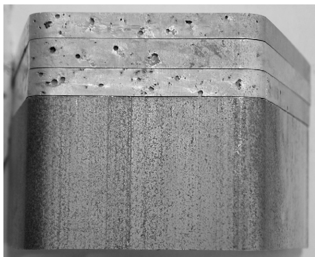
Fig. 1. Birds' view of the ZK60 bumper intended to be applied in a car, in which the three sections at the top are the cut samples after a salt spray test. The orientation of the component from bottom to top corresponds to the extrusion direction or the longitudinal direction (indicated by surface scratches).
